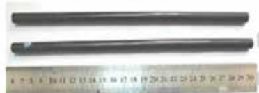
SiC/SiC 2 composite tube
